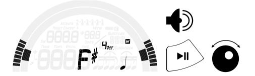
Any pitch, either detected in Auto Pitch Detection Mode or selected via Manual Pitch Selection, can be immediately heard by pressing the Play / Pause Button to enter Tone Generator Mode. The active pitch will immediately begin to play through the on-board speaker and the tuner will automatically switch to Manual Tuning Mode in order to allow for the adjustment of the sounding pitch by use of the Value Wheel.
